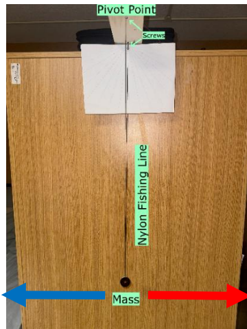
Fig. 1. Final construction of the pendulum. Angles were traced onto the white paper shown to allow experimenters to release the mass from the same reference point in each trial. Direction for positive (red arrow) and negative (blue arrow) angular displacement is shown.
