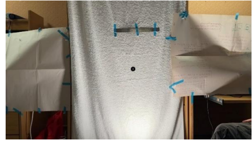
Fig. 2. A white background was added behind the pendulum to facilitate auto-tracking. This image also shows the direction in which Q factor was measured.
